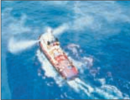
Sea trial off Gabon, West Africa; dispersant is being applied from a boat to a light crude oil, at an application ratio of about 5–10 per cent.
